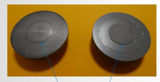
On the left: Pure niobium after 2000bar On the right: Anodized aluminium 7049A T6 after 5800bar
