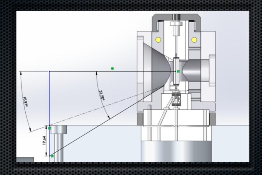
Scattering angle cut by stopped-flow system
