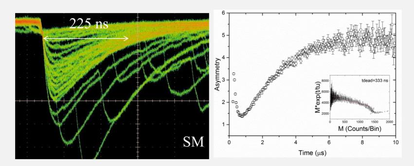
The situation is greatly improved by signal processing. Differentiated signals are shown with the corresponding improvement in the asymmetry plot.
