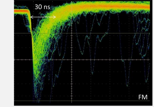
To characterise dead time performance, μSR spectra were recorded at various count rates typical for μSR experiments.
