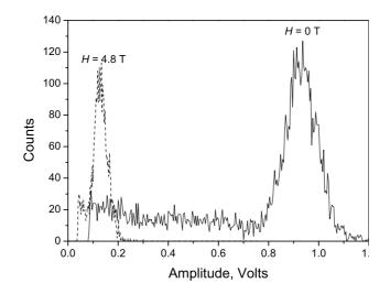
Figure 1: Amplitude distributions of the HAPD signals in zero and 4.8 Tesla magnetic field.
