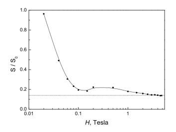
Figure 2: The change of the HAPD effective photosensitive area S with the magnetic field H ( $S_0$  is the photocathode area). The dashed line corresponds to 0.140 – the ratio of the APD to the photocathode area. The solid line is drawn to guide the eye.
