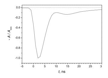
Figure 3: The averaged shape of the HAPD output pulse at H = 4.8 Tesla. The rise time is 2.0 ns. The pulse shape is the same as in zero field.
