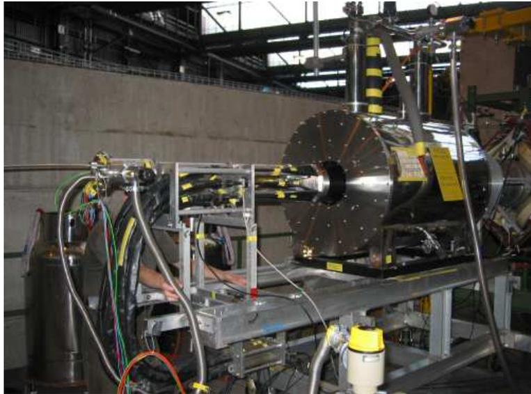
Figure 7: The ALC instrument at PSI, with the backward detector array and cryostat being inserted into the bore of the superconducting magnet.
