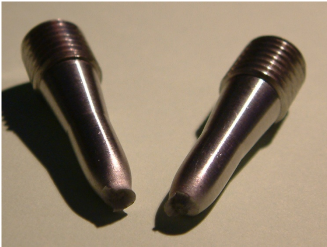
17-4PH tensile test sample
