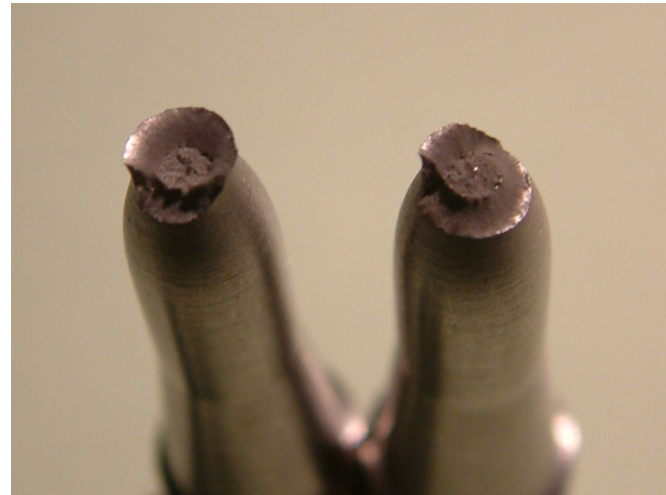
17-4PH tensile test sample
