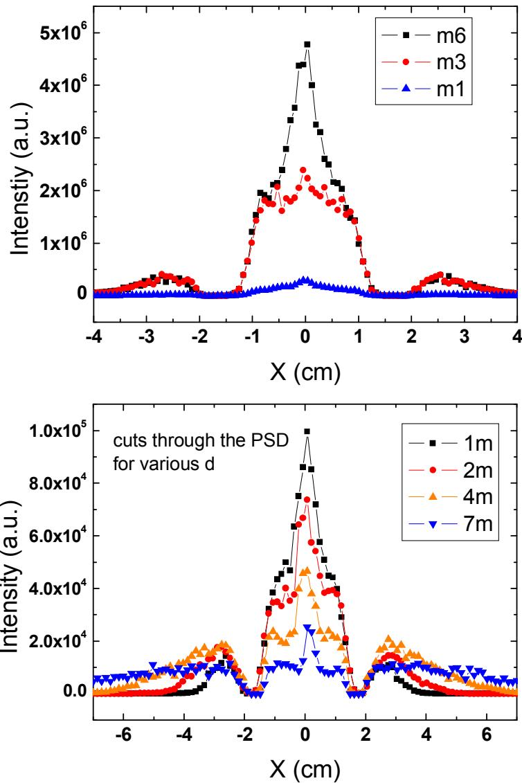
Intensity increases with increasing m value of the coating due to reflection of neutrons with higher angle of incidence
