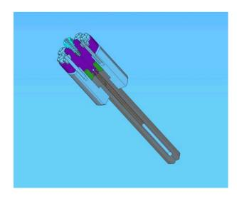
Following ISIS high pressure engineering practice the design pressure of the cell has been set up at **4.4 kbar** at **700K**. After manufacturing and assembling, the cell has been successfully tested up to **5.835 kbar** of hydrogen gas pressure at **20°C**, which, according to engineering model, should satisfy design pressure requirements at **700K**.
