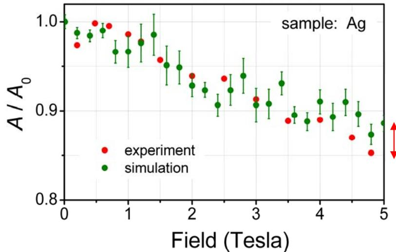
Relative change of asymmetry  $\sim 0.05$  at 4.8T is consistent with the time resolution of  $\sim 90$  ps, which is not considered in the simulation.
