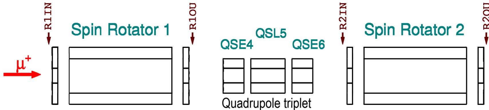
Spin Rotator – rotates the muon spin from “longitudinal” to “transverse” direction
