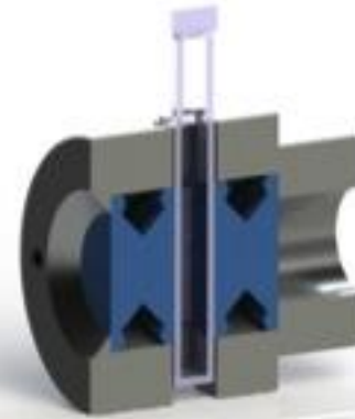
4 windows + sample in quartz cell
