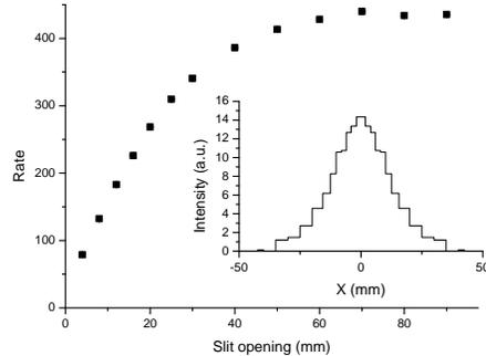
Figure 2: Measured rate in the MuSR instrument as a function of the collimation slit opening width. Inset: reconstructed beam profile at the slit position, assumed symmetric.
