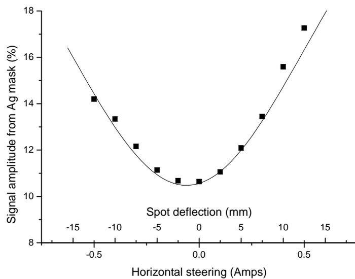
Figure 3: Typical horizontal steering curve from the MuSR instrument, with the spot (slits=8) moved across a 20mm Fe<sub>2</sub>O<sub>3</sub> sample. Runs 23861–71.
