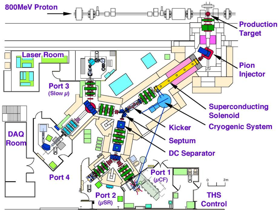
Figure 1: Layout of the RIKEN-RAL beamlines at ISIS, which can produce either decay or surface muons.
