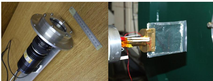
Figure 9: (a) The HiFi camera, lens and window. (b) The scintillator
