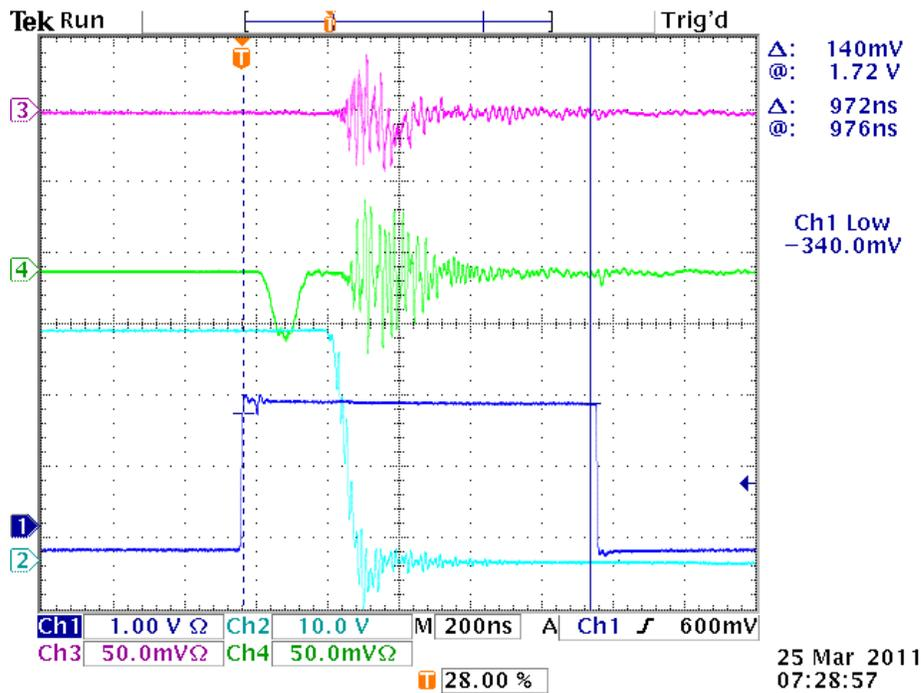
Figure 6: Monitoring signals from the ISIS kicker. From top, Ch3: Slit counter signal from the MuSR beam taking the second muon pulse (coincident with high frequency electrical noise). Ch4: Slit counter from EMU showing the 1st pulse. Ch2: Monitor voltage from the kicker electrode (scaled  $\times 10^{-3}$ ). Ch1: Trigger pulse.
