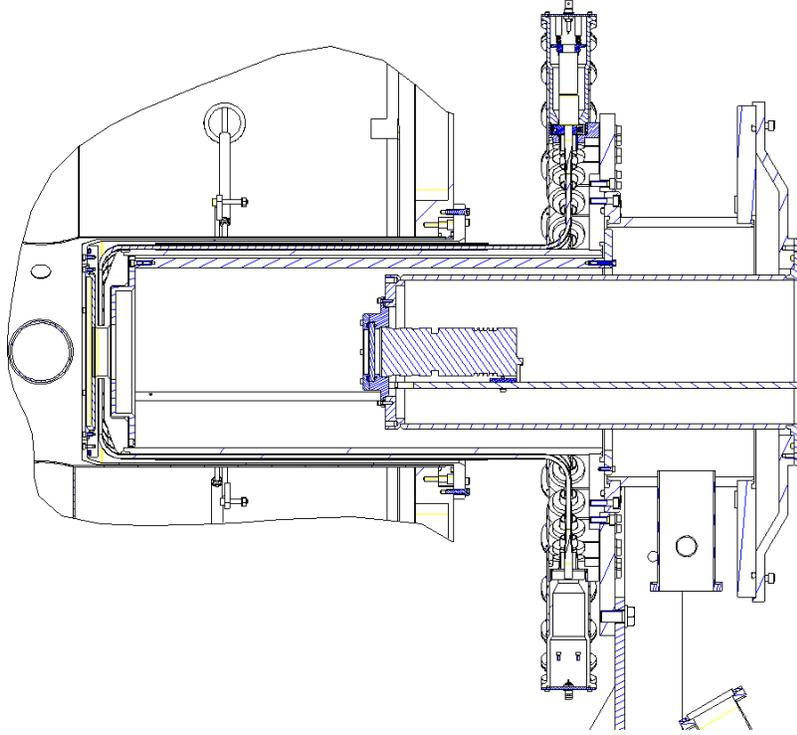
Figure 8: Drawing of the HiFi beam camera in position in the instrument. The CCR with scintillator is inserted through the magnet side port, shown end-on at the left.
