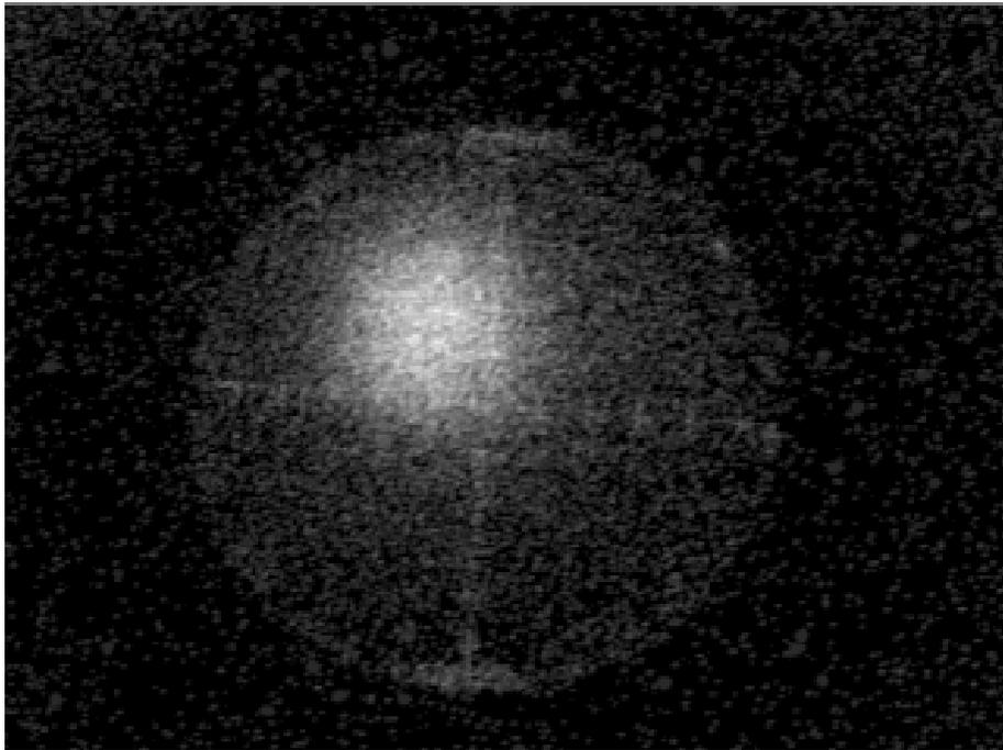
Figure 7: Averaged beam spot picture from the Eaton camera
