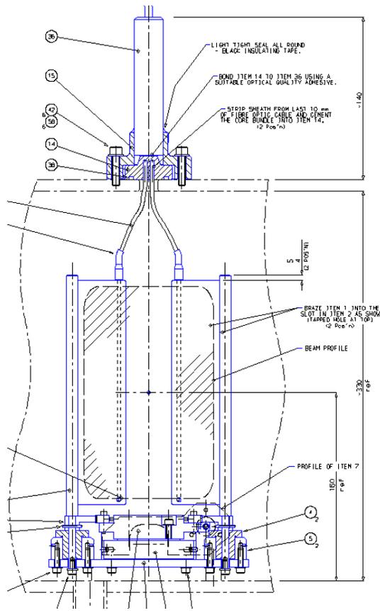
Figure 4: Drawing of the ISIS EC slit assembly, with scintillating fibres fixed to the edges of the slits.
