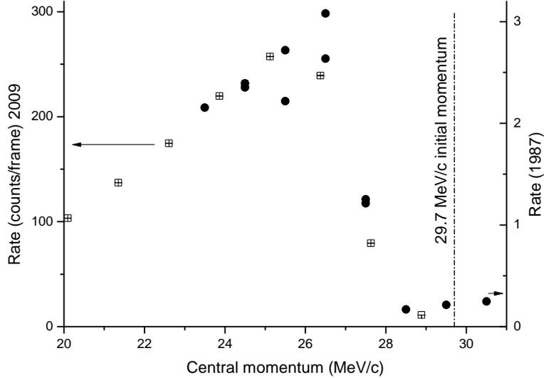
Figure 5: Momentum scan measured on the MuSR beamline at ISIS, by varying the fields in all magnets. Two data sets shown, taken in 1987 (when commissioned) and 2009. The cutoff is lower than the initial 29.7 MeV/c because of a thin Al window between proton and muon beam lines.
