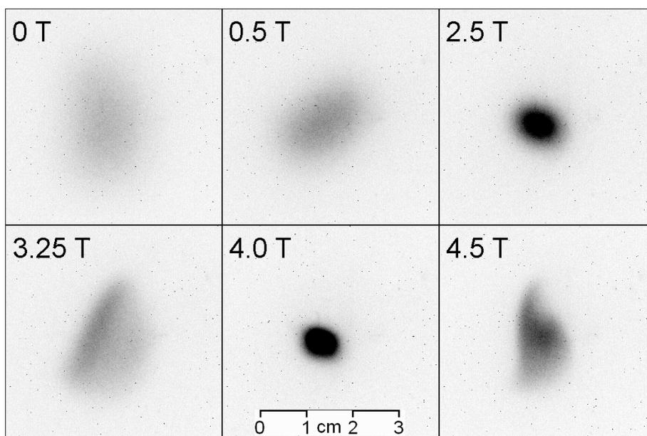
Figure 10: Typical beam pictures from HiFi at different magnetic fields
