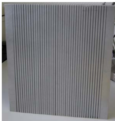
Fig 8. The first coil cut in Aluminum by electrical discharge machining.
