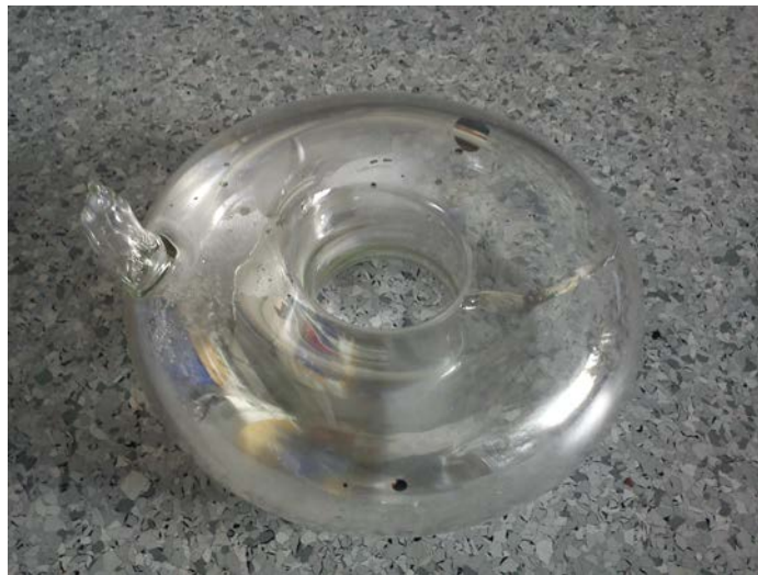
Fig.2. The first in the world doughnut shaped cell: outer diameter about 20cm.
