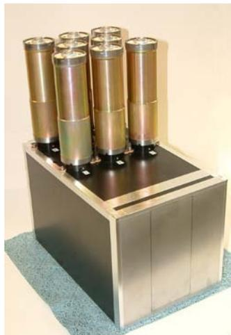
**Figure 23:** *Photograph of the detector mechanics that has been constructed for evaluating the LGBO scintillator in a 27 element linear detector with a 3 mm position resolution*
