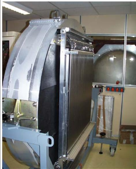
*Front view of the detector showing the 128 PSPC mounted on their frame.*
