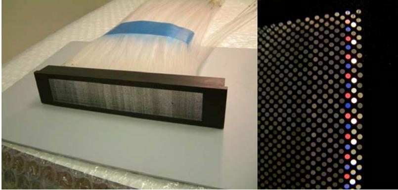
*Figure 18: Two photographs of the fibre block of the 1.2 mm prototype detector. The photograph on the left shows the B<sub>4</sub>C block with the 6000 optical fibres. A close up of the fibre block, demonstrating the fibre arrangement, is shown on the right.*
