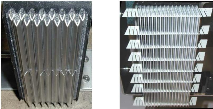
***Figure 3: Pictures of the front end of the prototype detectors with the so-called “V” geometry on the left and the “Venetian” geometry on the right.***
