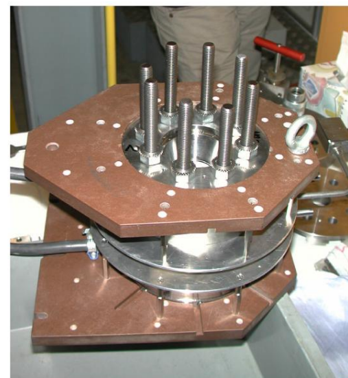
Hydraulic cylinder for biasing the window
