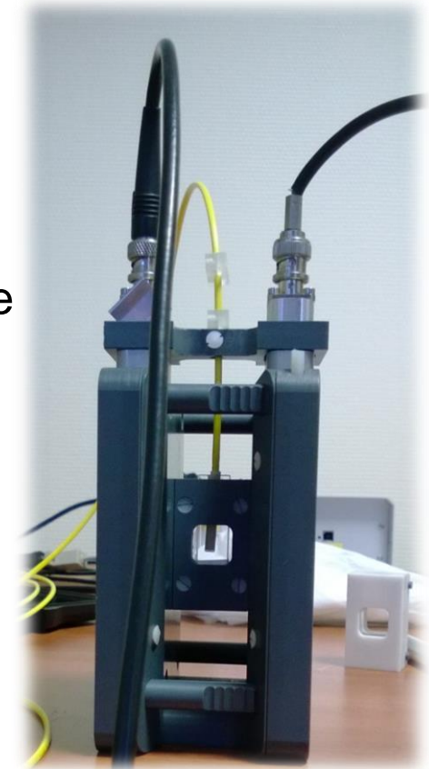
Sample holder in PVC on the EFC and the sample holder in PTFE (behind)
