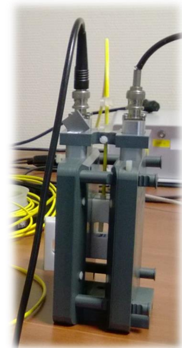
Electric field cell in the 25mm space configuration
