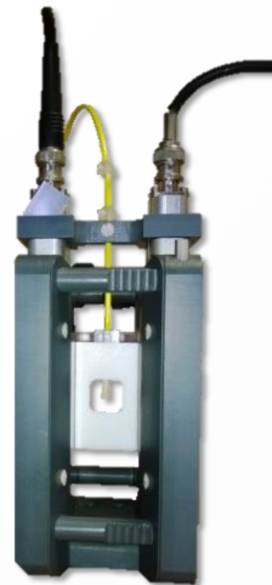
Kapteos probe inside an Hellma® cell
