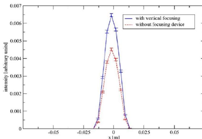
Fig. 1: Comparison of peak resolution/gain with and without vertical focusing device
