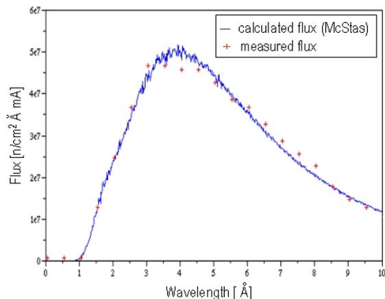
Fig. 3: Available wavelength spectrum at the TASP monochromator position; comparison of calculated and measured spectrum
