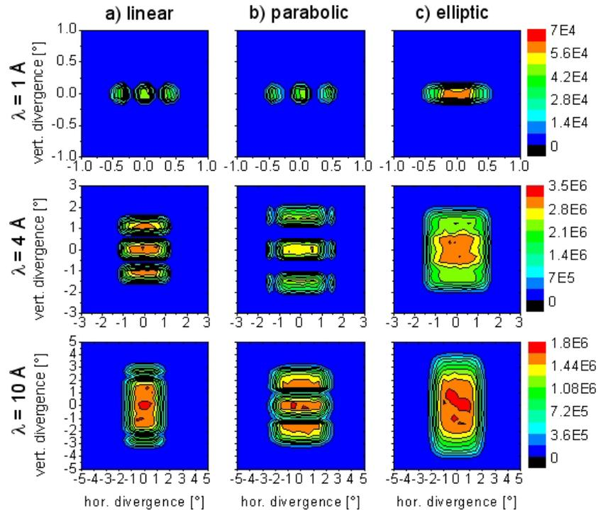
Fig. 7: Vertical and horizontal intensity distribution versus the divergence for wavelengths  $\lambda = 1 \text{ \AA}$ ,  $4 \text{ \AA}$ ,  $10 \text{ \AA}$  of a) ballistic guide with linearly tapered divergent and convergent sections, b) ballistic guide with parabolic divergent and convergent sections, c) elliptical guide.
