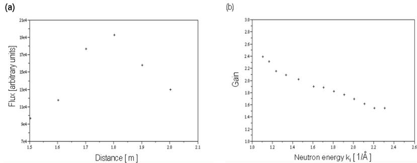
Fig. 5: (a) neutron intensity behind guide exit – focal point at 1.8 m after monochromator;
