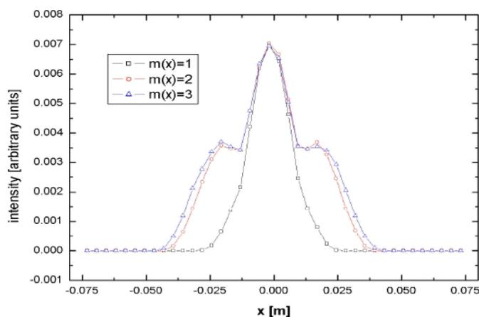
Fig. 2: Comparison of peak resolution for different reflectivity values of the vertical walls
