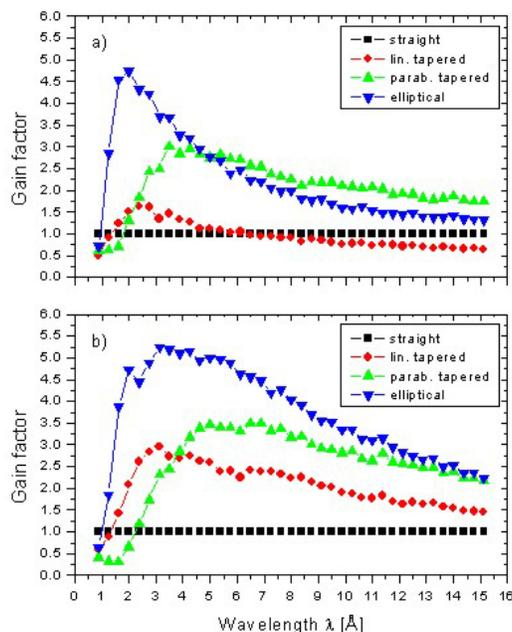
Fig. 6: Gain factors of various guide geometries normalised again a straight supermirror guide ( $m = 2$ ). Gain factors are calculated from integrated intensities (10 x 40 mm<sup>2</sup>) at a distance of a) 1.3 m and b) 0.5 m from the guide exit.
