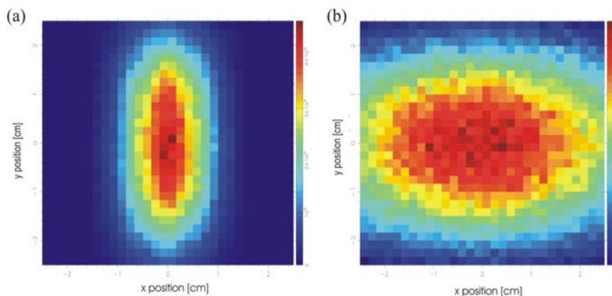
Fig. 4: Comparison of the beam spot at the sample position; (a) with vertical/horizontal parabolic trumpet; (b) without trumpet
