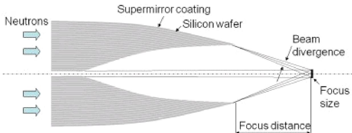
Such focusing lenses can be used for imaging purposes where i) cone beam geometry is used or ii) high-flux density in the focal point is used for high-spatial resolution experiments.
