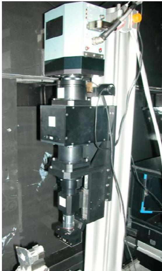
**High-resolution neutron imaging setup. A Kumakhov lens is used to focus the beam at the scintillator screen. High resolution detector based on light microscope magnifies the image from the scintillator on the CCD chip providing effective pixel size of 2  $\mu\text{m}$ . The setup was equipped with a GGG scintillator screen.**
