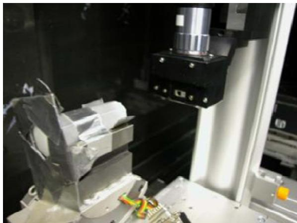
**High-resolution neutron imaging setup. A Kumakhov lens is used to focus the beam at the scintillator screen. High resolution detector based on light microscope magnifies the image from the scintillator on the CCD chip providing effective pixel size of 2  $\mu\text{m}$ . The setup was equipped with a GGG scintillator screen.**
