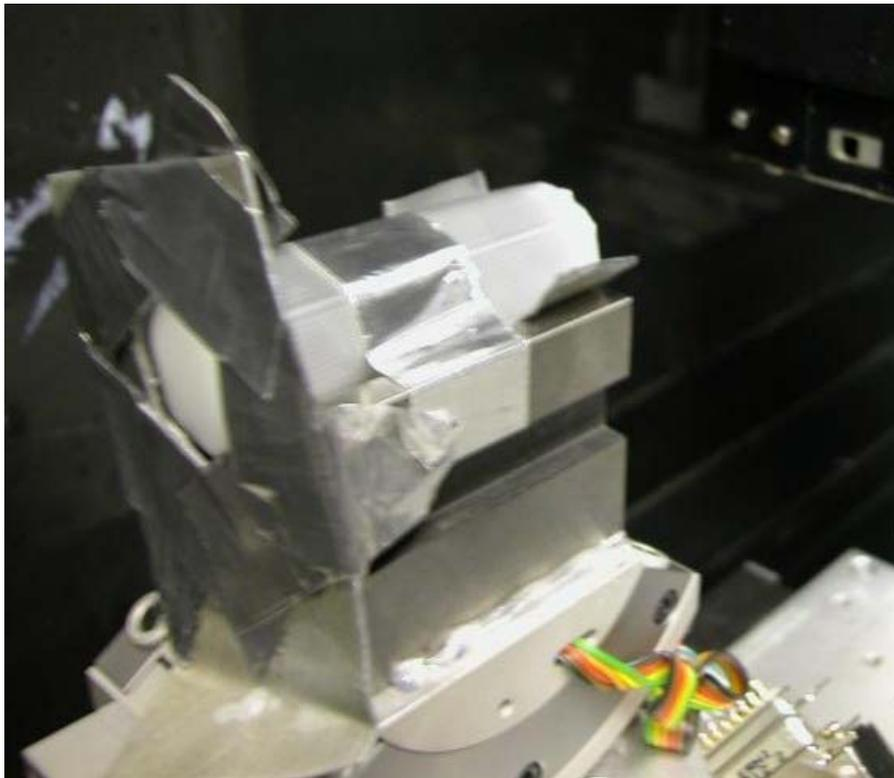
**A focusing device based on Kumakhov-type lenses was used which focuses a cross-section of 2 cm into a diameter of less than 1mm provided a flux gain of 20x which was essential for the application of a high resolution detector with a pixel size of 2  $\mu\text{m}$ . In this way realistic exposure times of several minutes were achieved.**
