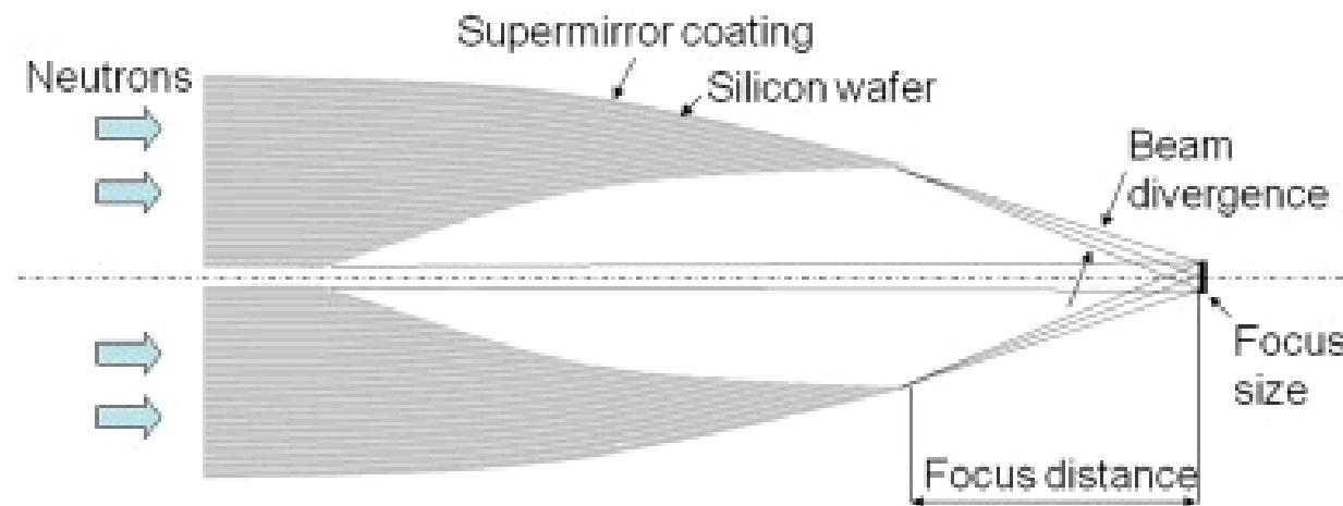
Such focusing lenses can be used for imaging purposes where i) cone beam geometry is used or ii) high-flux density in the focal point is used for high-spatial resolution experiments.
