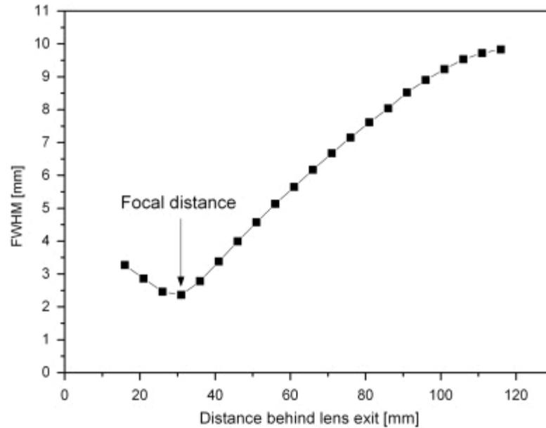
**FWHM of the neutron intensity perpendicular to the beam direction in dependence of the distance from the end of the lens.**
