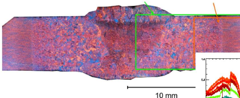
**Zr-alloy weld: different grain structures result in large differences in transmission spectrum**
