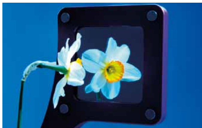
Figure 1. (Left) A mirror consisting of a \text{Mg}_{0.7}\text{Ti}_{0.3} thin film. (Right) After applying a hydrogen containing gas, the mirror changes into a light absorbing \text{Mg}_{0.7}\text{Ti}_{0.3}\text{H}_x film.
