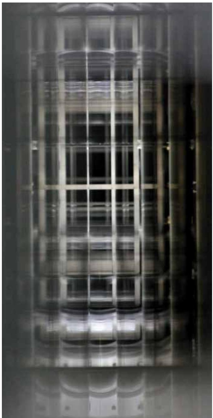
BioRef is a newly built time-of-flight reflectometer at the Helmholtz-Zentrum Berlin dedicated to biological samples. View from the sample position of the time-of-flight reflectometer BioRef through the guide system of the instrument.
