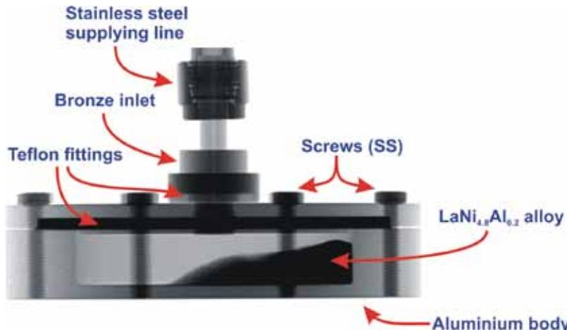
Figure 2: Radiographic image of the investigated container. All details of the construction are excellently visible.
