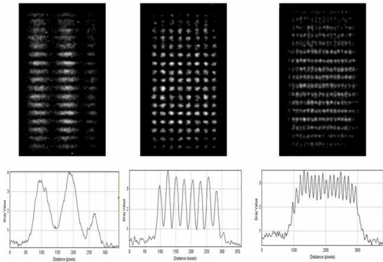
Figure 1: Modulation patterns measured at the monochromatic SESANS instrument at RID with an imaging detector system from the beamline CONRAD at HZB [9] for different magnetic field settings. Note that the horizontal stripes only display the structure of the used polarisation analyser.
