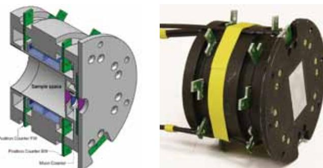
Figure 5: A prototype detector module based on avalanche photodiodes developed at the S $\mu$ S with schematic view shown on the left.
