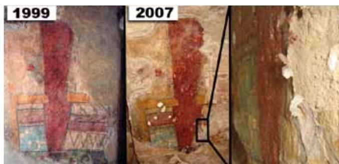
Figure 1: The picture shows a Maya wall painting coated in 1999 with a film of Mowilith DM5 (vinyl acetate/n-butyl acrylate 65:35 copolymer). In less than ten years severe loss of pictorial layer occurred. The right box shows the powdering of the mortar promoted by the action of salts, which are forced to crystallize behind the surface due to the presence of the polymer coating.
