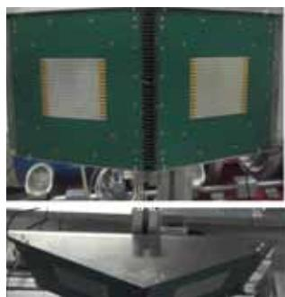
Figure 2: Triangular magnetic field regions for the TOF SEMSANS experiment at WESP at RID
