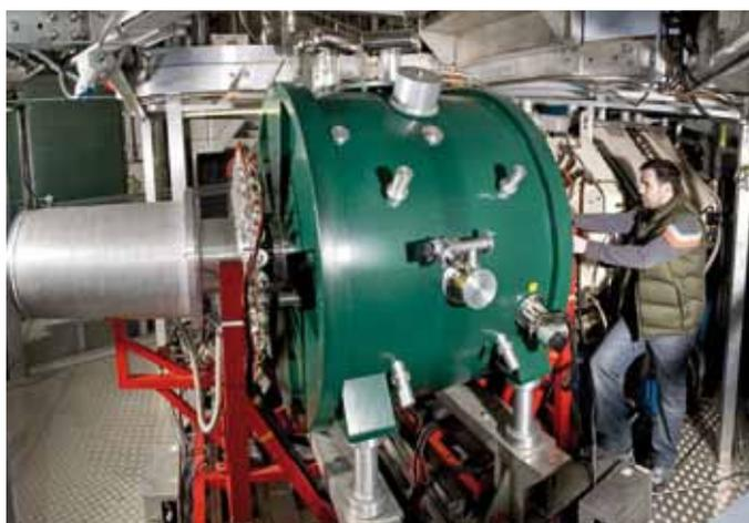
The new high-field muon spectrometer (HiFi) at ISIS provides magnetic fields up to 5T for muon studies of magnetism, molecular dynamics and polymer systems. Computer simulations of muon and positron paths through the instrument were undertaken with NMI3 JRA funding to enable the instrument detector array to be designed. The instrument is working very successfully as a full part of the ISIS user programme.
