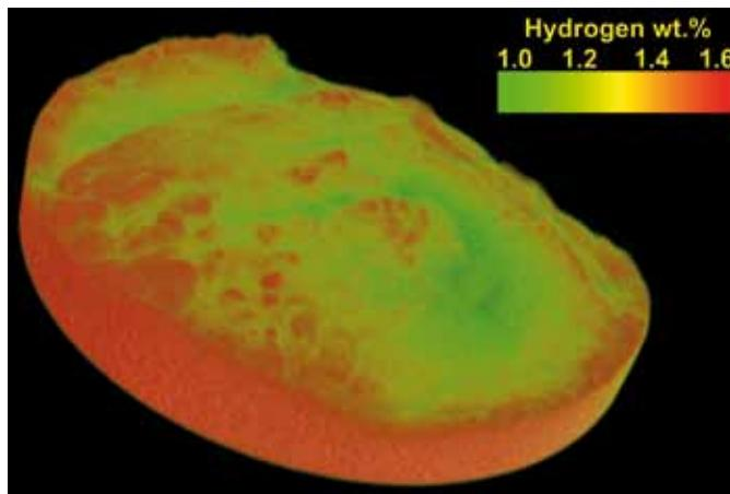
Figure 3: The interior of the hydrogen storage container, only the bed without details of the container is displayed. Different colours represent the hydrogen concentration in the bed: green means low hydrogen concentration, orange – high. As apparent, the concentration is enhanced around walls.
