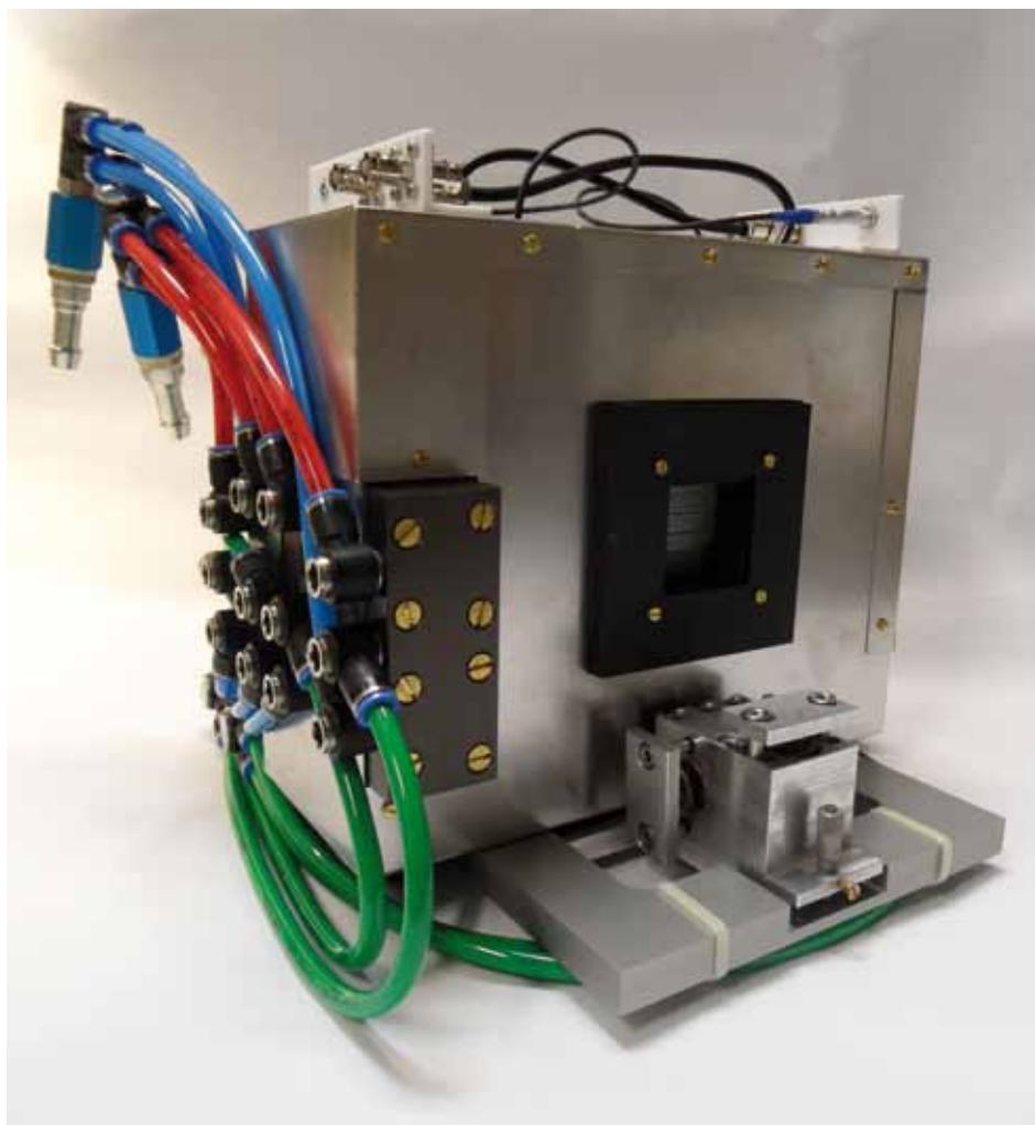
New spin-flipper for neutron resonance spin-echo (NRSE) spectrometer MUSES at LLB, CEA-Saclay.
