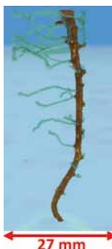
Figure 1: A three-dimensional representation of the roots of a chickpea plant. The image was obtained from segmenting the roots in the reconstructed neutron tomography data.
