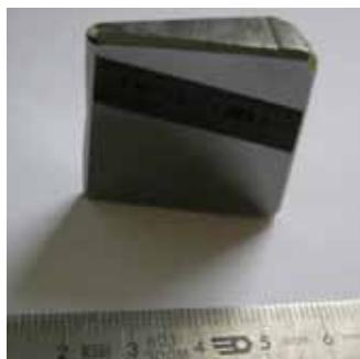
Figure 1: A prism made of TGG ( $\text{Te}_{78}\text{Ge}_{11}\text{Ga}_{11}$ ) glass.
