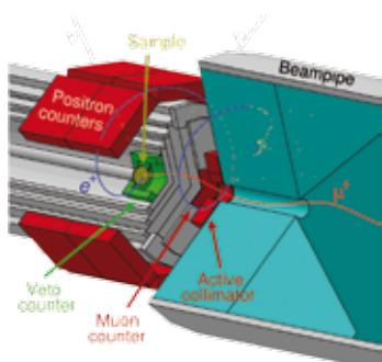
Figure 4: A study of the detector geometry and positron trajectories for the S $\mu$ S high transverse field spectrometer.
