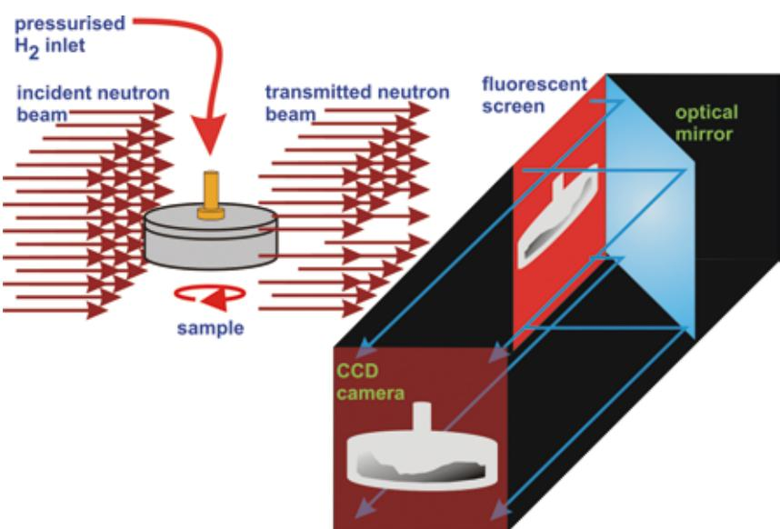
Figure 1: Experimental set-up. Schematic drawing presenting the configuration used for neutron imaging studies.
