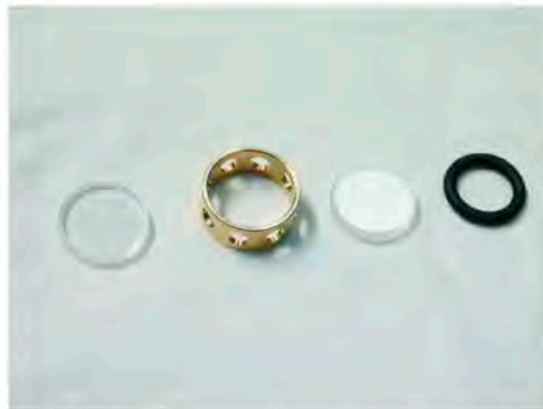
FIG. 4. (Color online) Components of the pill: the brass ring with holes on the periphery, the two sapphire plates, and the O-ring. The sample in the pill is sealed against the hydraulic oil when the two sapphire plates press the O-ring against the brass ring holes from inside.
