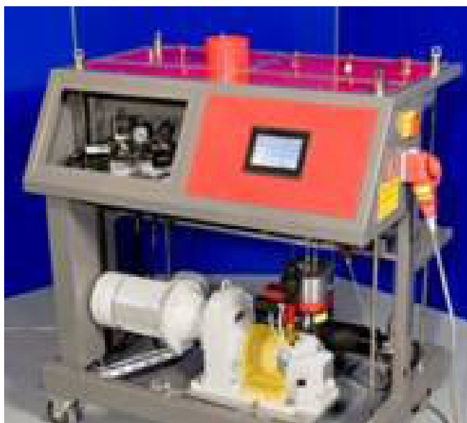
Fig 2. ISIS 10 kbar hydrogen gas intensifiers
