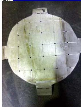
Cd mask with 1mm holes at 10mm pitch
