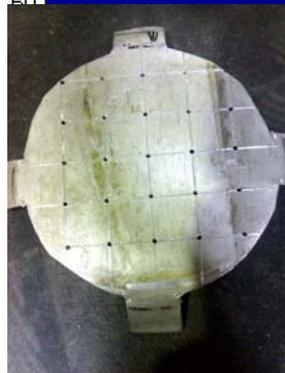
Cd mask with 1mm holes at 10mm pitch
