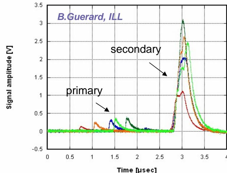
*PMT signals of primary and secondary light produced in a MSGC at ILL*
