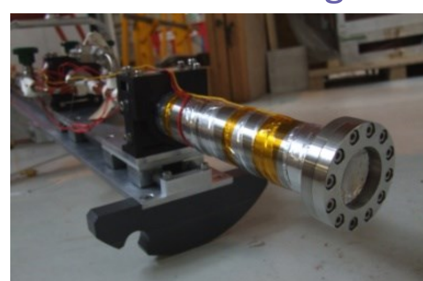
Gas target pressure cell designed for the ISIS high field spectrometer
