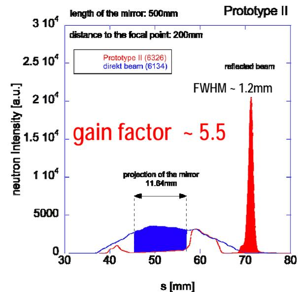
add on lens system for BOA to focus in 2 dim on samples of 5x5 mm
