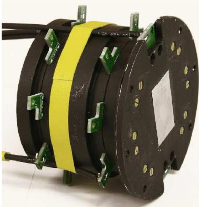
Figure 2: Prototype timing detector. The aluminized mylar window for incoming muons can be see in the front of the detector. Only 4 positron counters and the muon counter have been wired in this picture
