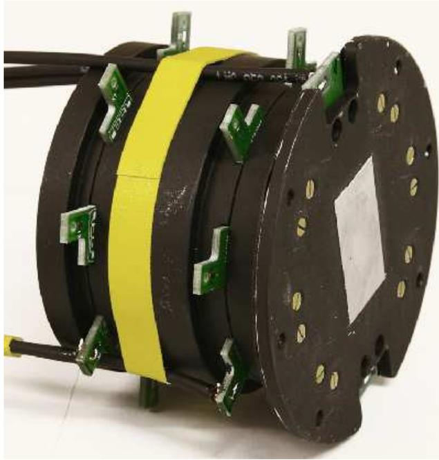
Figure 2: Prototype timing detector. The aluminized mylar window for incoming muons can be seen in the front of the detector. Only 4 positron counters and the muon counter have been wired in this picture
