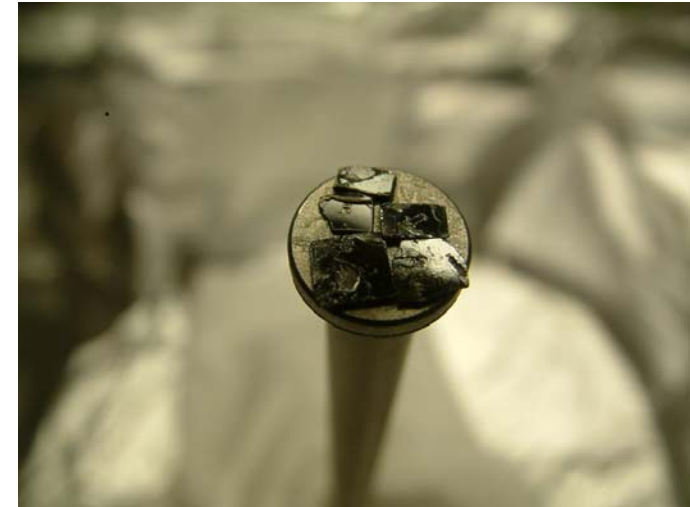
“untwinned” YBCO-7 Crystals ( from UBC R. Liang, W. Hardy et al.)
