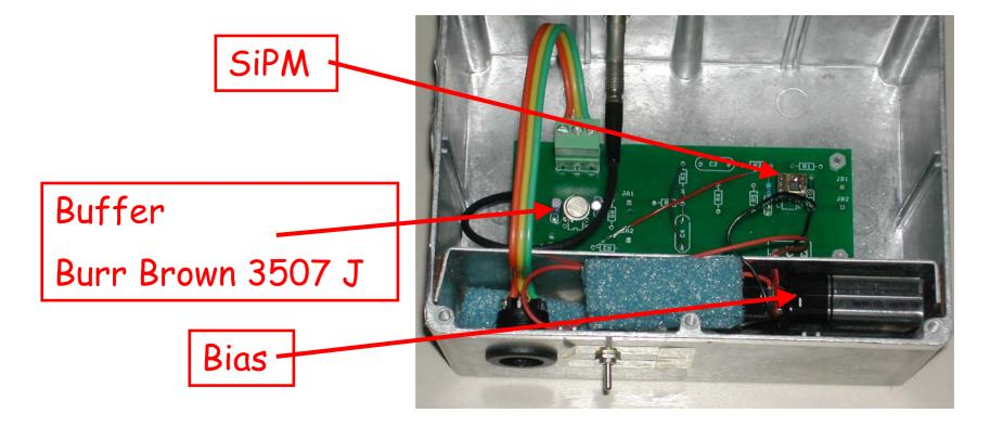
The SiPM is mounted on a small test board which can be removed to compare different devices.
