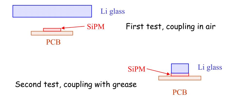
The second test was perfomed in similar conditions but the scintillator was small ( $3x3 \text{ mm}^2$ ) and coupled directly on the SiPM.
