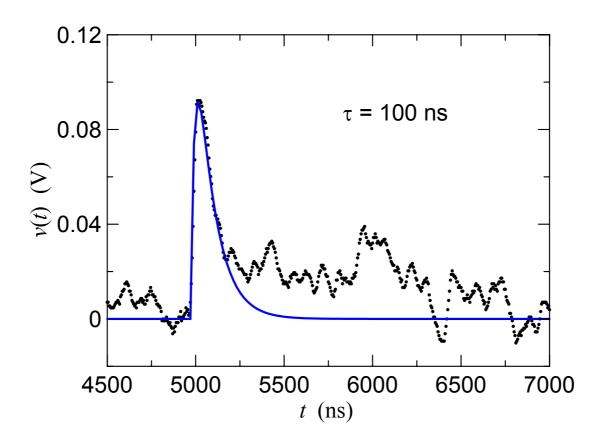
Similar results, but with longer decay time were obtained using a ZnS scintillator in a similar configuration. The time step was 5 ns, while the rest of the sistem is identical.
