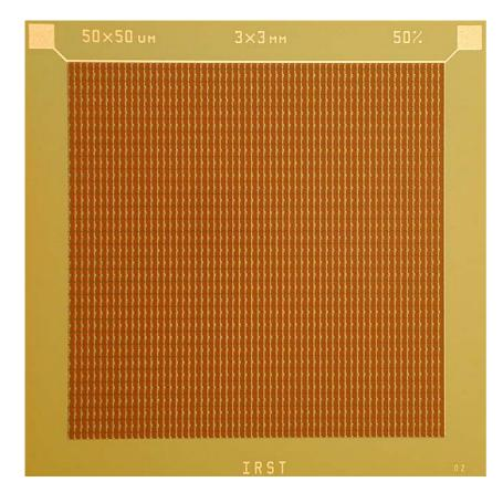
Width of the dead region around each micro cell, 50  $\mu\text{m}.$
