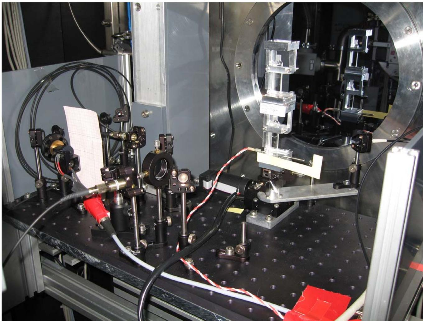
SLS data at KWS2 – goniometer configuration with rectangular cuvette - suitable for neutron scattering
