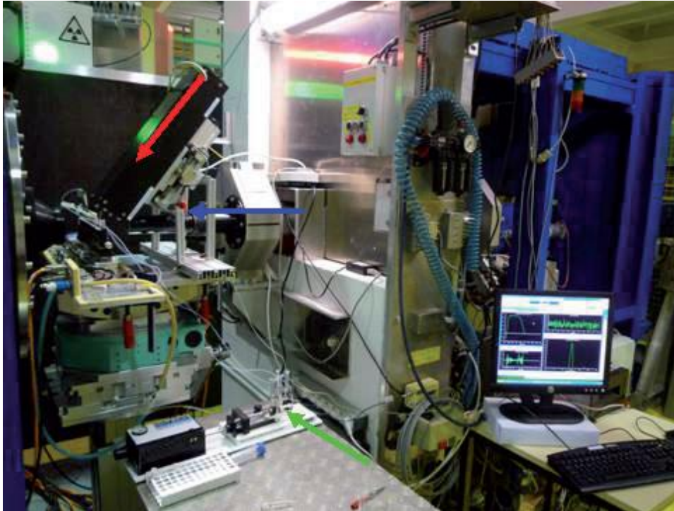
Figure 1: DLS-SANS set-up at D11 (courtesy of Th. Nawroth, U Mainz). The red arrow marks the incident laser light direction, the blue arrow the incident neutron beam direction and the green arrow highlights the stopped-flow mixing device.
