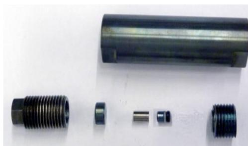
Figure 18. Up: Schematic view of the two-layer p-cell opened both side; Down: picture of the sealing system.
