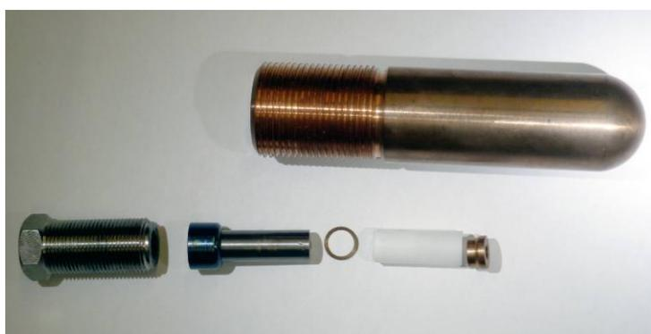
Figure 17. Picture of the sealing system for the p-cell opened one side.
