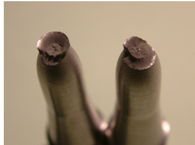
17-4PH tensile test sample
