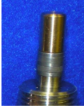
Double Bridgman seal prior to pressurisation.
