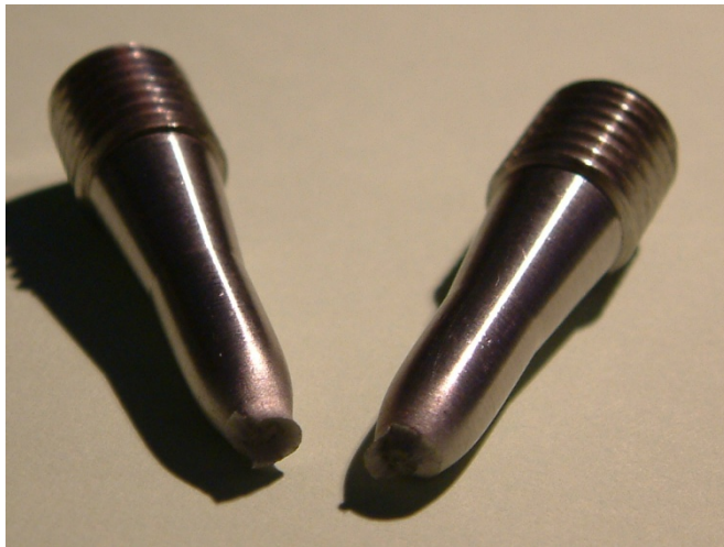
17-4PH tensile test sample
