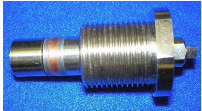
Typical Bridgman seal arrangement showing a three part seal assembly and the supporting backing nut.
