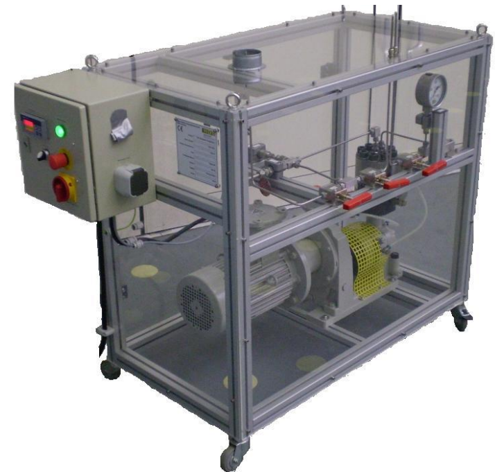
3 kbar hydrogen membrane compressor
